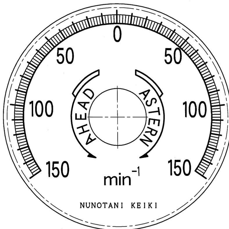
Propeller Shaft Revolution Indicator
