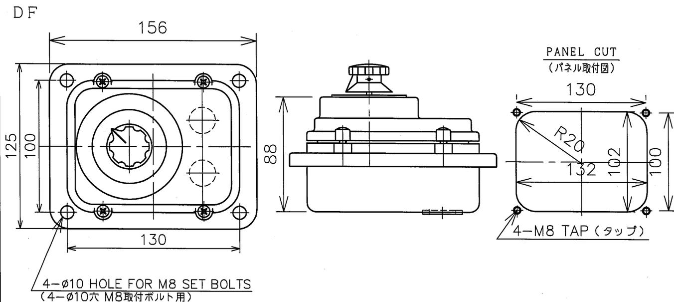
Propeller Shaft Revolution Indicator
