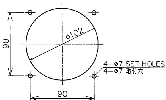
Propeller Shaft Revolution Indicator
